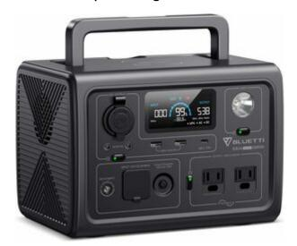
The negatives: The internal battery is 22V, so the 12V output is from a DC-DC converter and is limited to 10A. So when operating SOTA or POTA it's best to keep HF power under 50 watts. Also the USB-C doesn't seem to coordinate well with some devices,
