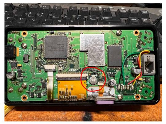
FTM-400 Display Panel. The Li-Ion backup battery is circled. 16 May 2022 we have a single photo. This is a commercial installation at a water tank @580 meters ASL in Escondido, CA. It seemed a rather unique and poor way to run the feed line. Not good to have the feed line up against the antenna. And who knew the antenna would tilt? Probably a good idea to run a more substantial support. Why not just mount the antenna to the pole?
