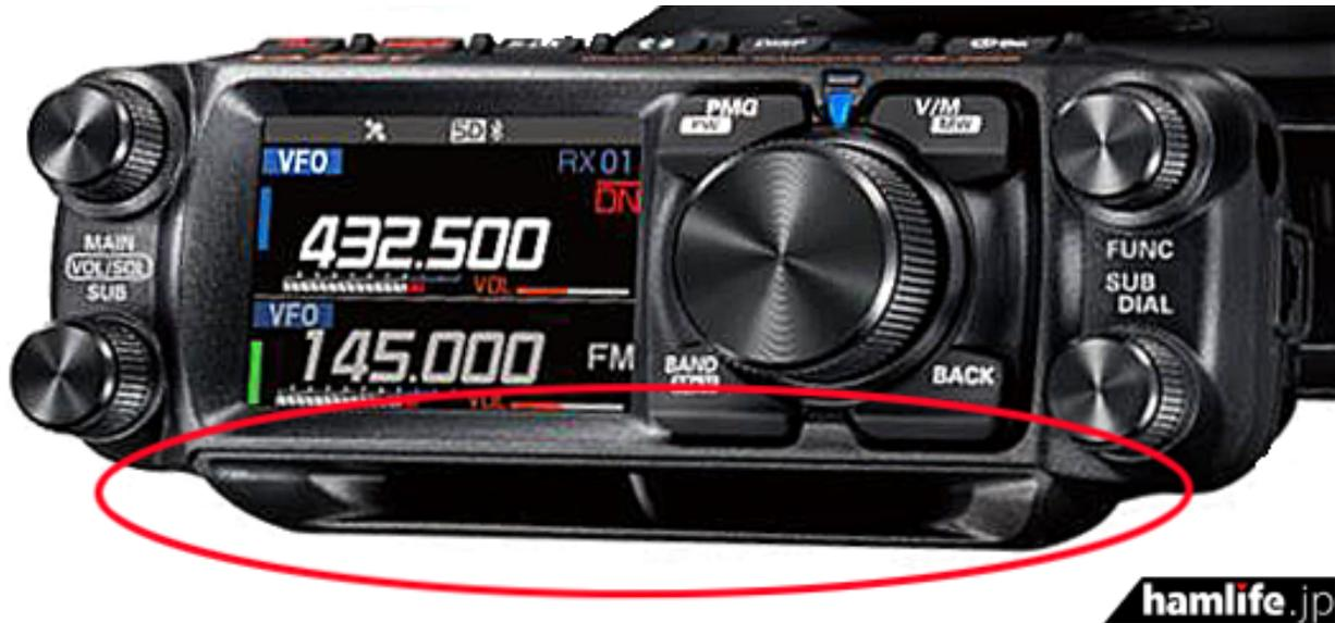
6W high-output front speaker built into the control head (image photo created by hamlife.jp)
